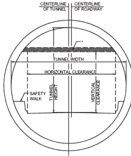
Figure 2.2: Circular tunnel with two traffic lanes and one safety walk (Source: Highway and Rail Transit Tunnel Inspection manual, 2005)
